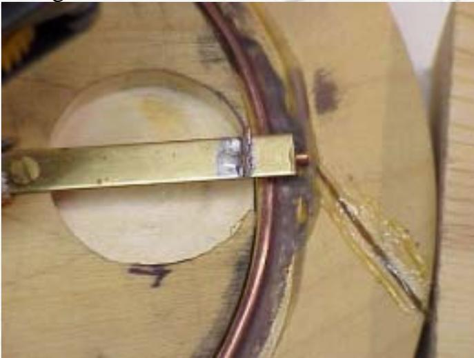
The above photo shows that the rotor, near the North magnet hole, only clears stator by about a 64<sup>th</sup> of inch (for reference, magnets are 1.125 inches in diameter).
